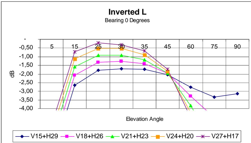
In this graph – the direction opposed to the horizontal wire – we see about 2 dB lower gain of the lower antenna compared to the highest one, until 45 degrees of radiation angle, where the situation is reversed.
