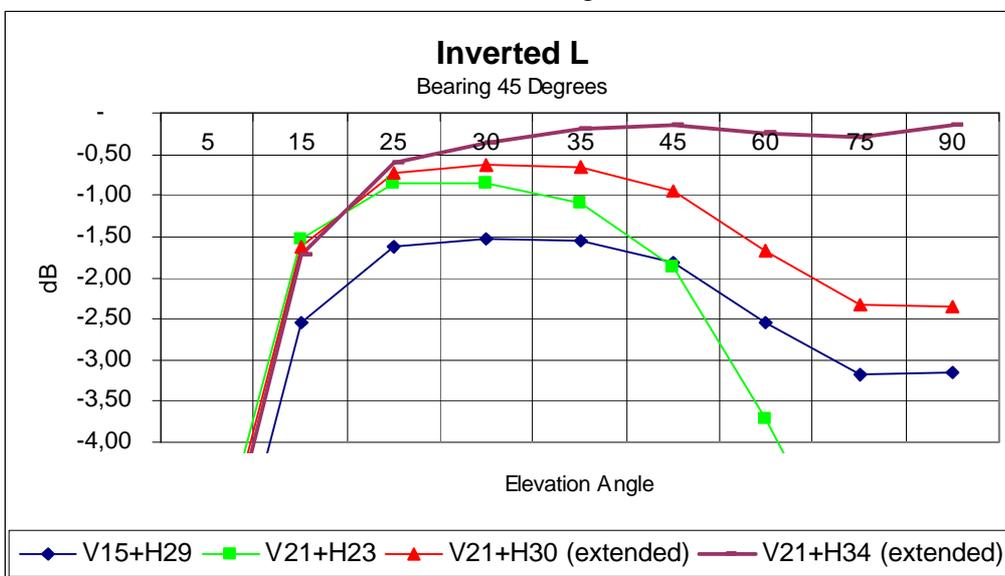
The 51m. antenna looks like the lower Inverted L, about 1 dB better, while the longest one is definitely a cloud warmer.
