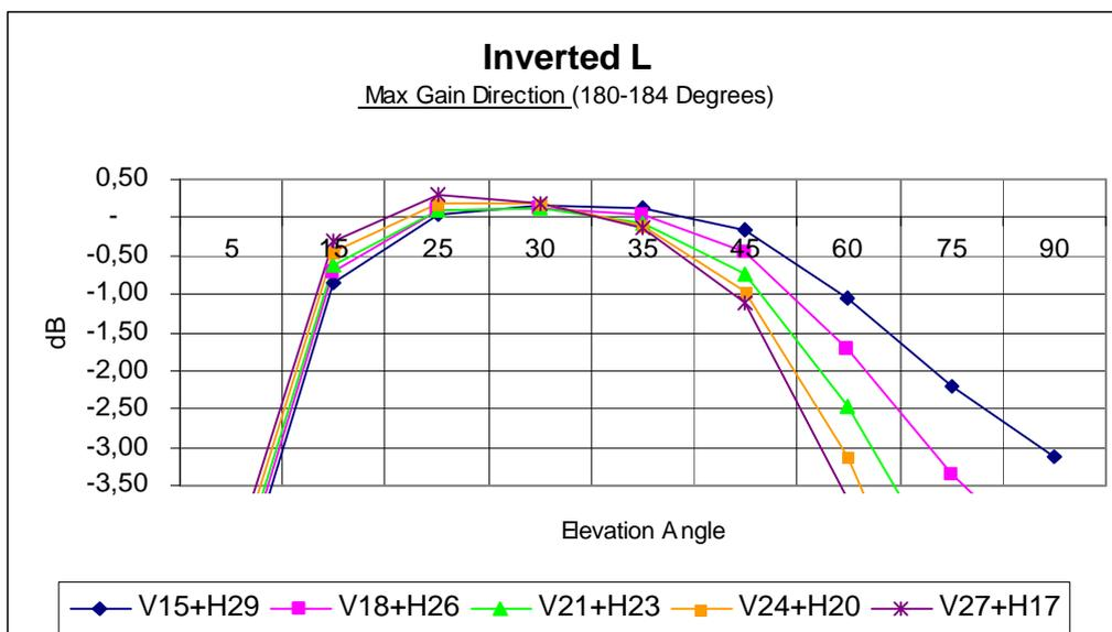
In this graph – the direction of the horizontal wire – we see a small gain of the higher antenna at low angles, no difference at 30 degrees, and a much more high angle radiation by the low antennas.
