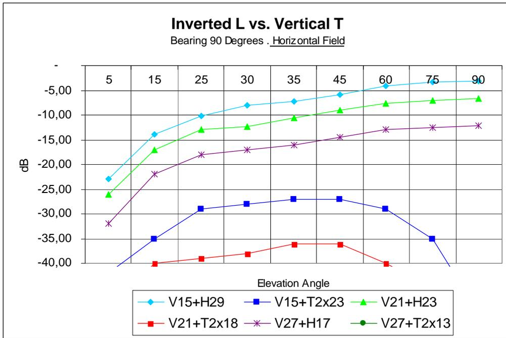
The best antenna on this graph appears to be the lowest one (with longest horizontal wire), but we saw above that it wastes too much energy on higher angles. T verticals are at least 25dB down or out of picture.
