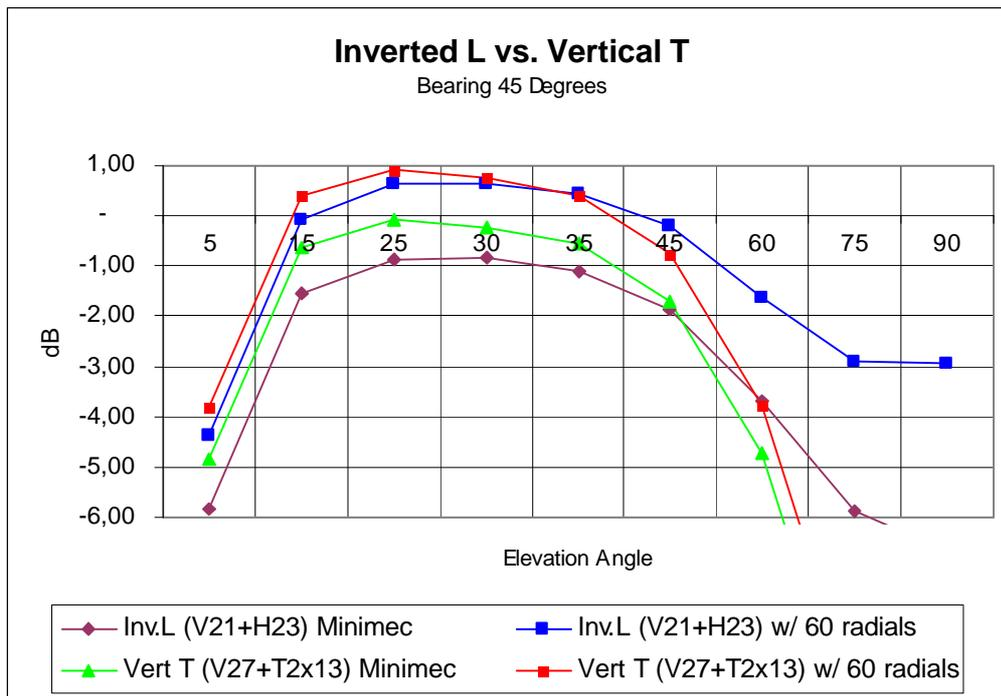
They look quite well also with the real ground and this graph definitely confirms that the Vertical T is better for DXing at our mid-latitudes and high-latitudes, but for low-latitudes, where higher radiation angles and horizontal polarization are needed, this inverted L should be used.
