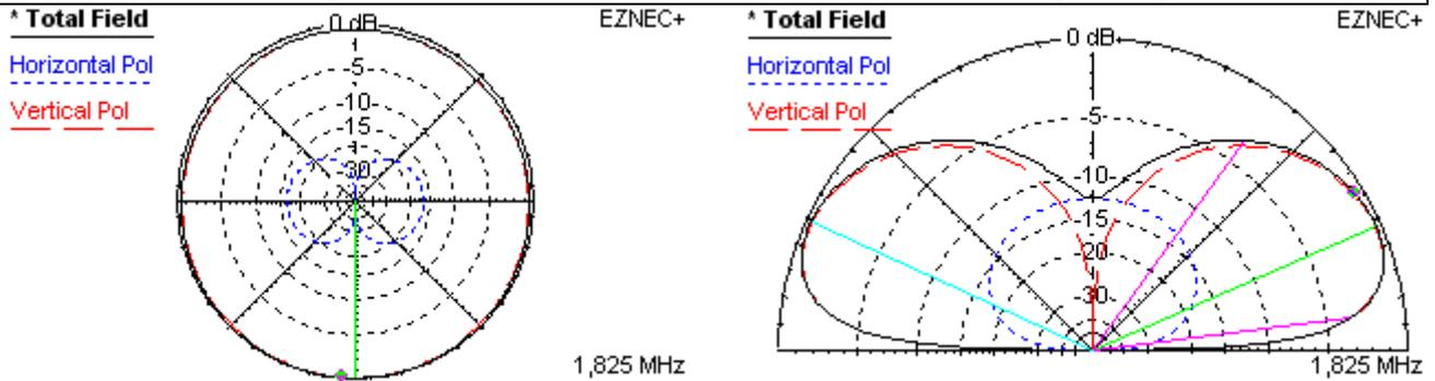
Azimuth and elevation plots for the highest Inverted L (V27+H17) – bearing 90 degrees
