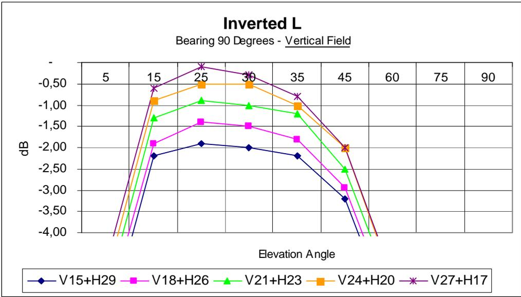
The vertical field holds up at low angles, but it's about half dB lower than the total field, meaning that there is also a small contribute from the horizontal component.
