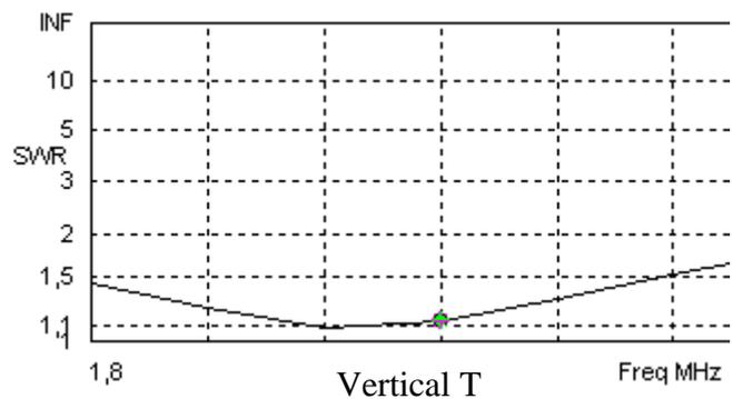
As expected, the vertical T is little broader the inverted L, but both are perfectly matched to the 50 ohms feeding line by means of easily manageable components with low losses.
