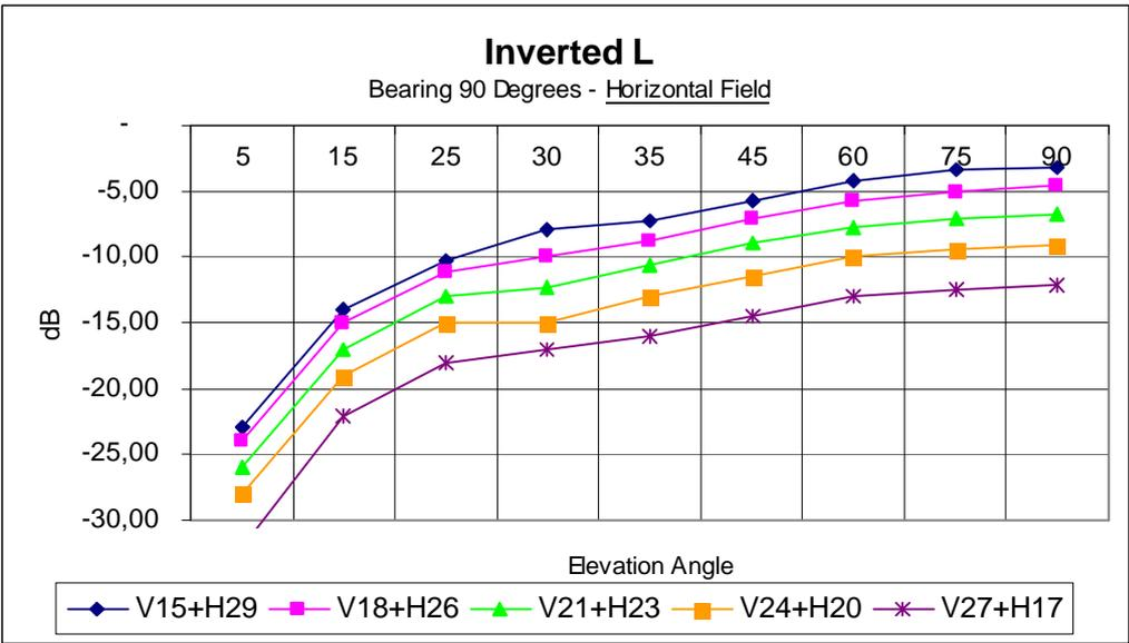
This is the horizontal field which, at low elevation angles, is more than 10 dB down, but at high angles becomes relevant, especially for the longer horizontal wire antennas.
