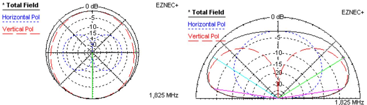
Azimuth and elevation plots for the lowest Inverted L (V15+H29) – bearing 90 degrees
