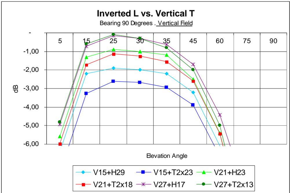
The vertical field at 90 degrees bearing is almost the same from both antennas 27m. high; there is a small difference at 21m., while lowering at 15m. it's better the inverted L than the vertical T.
