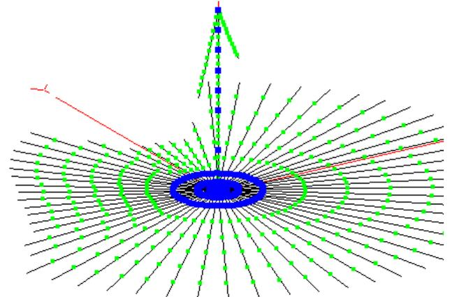
Vertical T (27m. high + 2 x13 loading wires)
