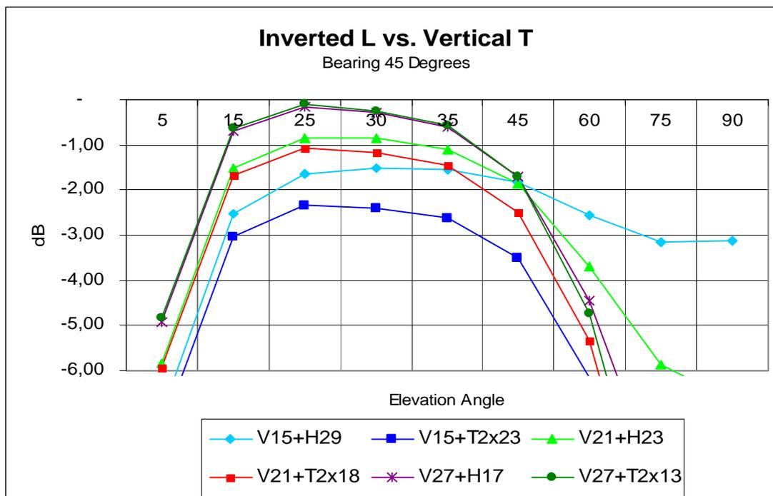
Bearing to Europe: at 27m. height there is no difference between Inverted L and Vertical T; at 21m. the inverted L seems better. The 15m vertical T loses even on high angles, but the inverted L has too much high angle radiation
